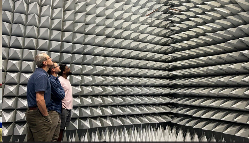
Inside the Anechoic Chamber of the Applied Research Building (ARB).
